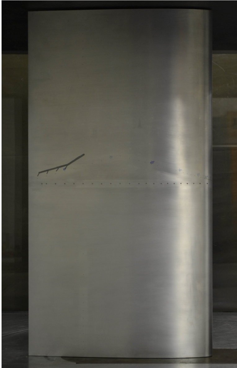
Fig. 3.3 Clean NACA 0012 airfoil model installed in the wind tunnel test section.
