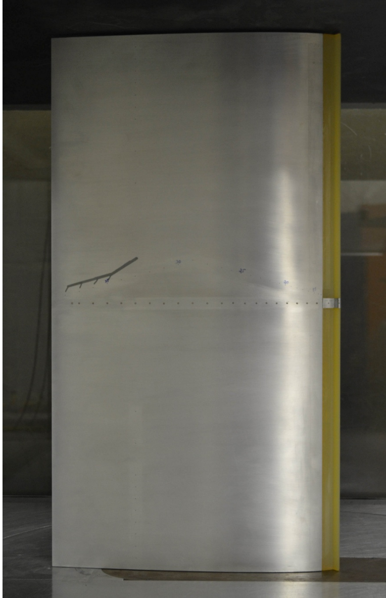
Fig. 3.5 Iced NACA 0012 airfoil model installed in the wind tunnel test section.
