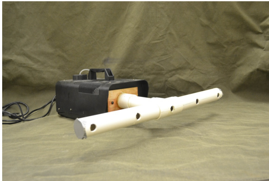
Fig. 3.23 Fog machine with PVC attachment used for smoke flow visualization.
