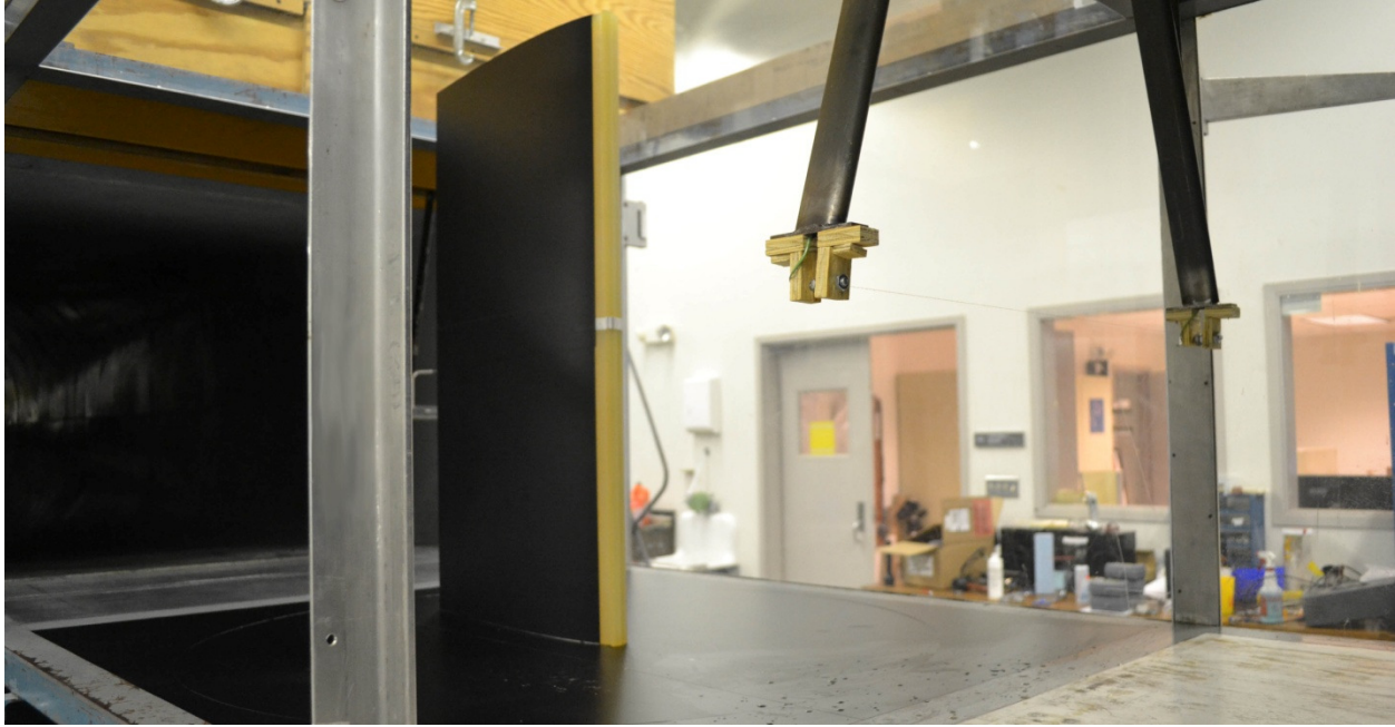
Fig. 3.24 Smoke wire and support structure installed upstream of airfoil model (view angled downstream).
