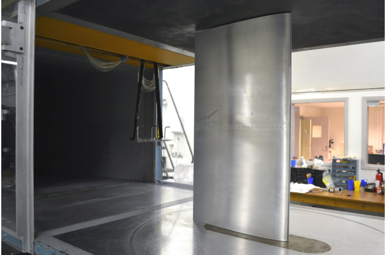
Fig. 3.10 Wake rake installed in test section downstream of NACA 0012 airfoil model.
